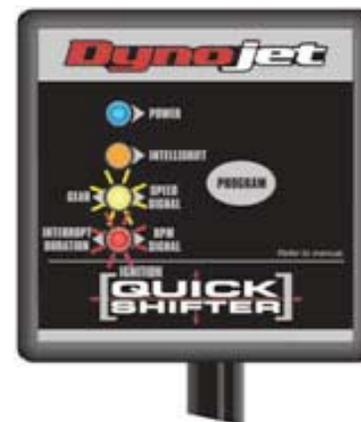
**Note2:** (If the Red interrupt duration/RPM signal LED does not flash in unison with the engine then the engine does not have a suitable RPM signal, you must now cut the thin black tacho signal sensing wire at the ignition coil connector and pull this wire back through the loom where it loops out of the loom, it might be tough to pull through but it will go, now connect it to the bikes original tacho signal wire. This wire normally runs directly from the bikes ECU to the back of the gauges.
