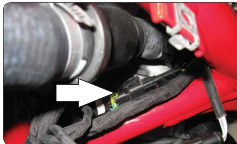
Figure C: Rear coil connection
