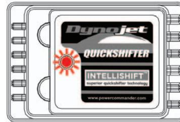
Move the gear lever to the trigger position 4 times, you'll see the status LED momentarily change to GREEN when the sensor is in the trigger position, then release the gear lever. Once you have moved the gear lever to the trigger point 4 times you'll now be able to count 14 RED status LED flashes. By doing this you'll have increased the interrupt duration in RPM Band#2 by 8ms. (Remember, each RED status LED flash is worth 2ms)
