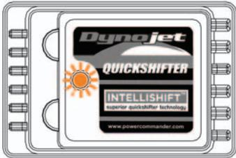
Move the gear lever to the trigger position once, you'll see the status LED momentarily change to GREEN when the sensor is in the trigger position, then release the gear lever. You'll now be able to count 6 ORANGE status LED flashes. You can repeat this action up to a maximum of 15 flashes and back to a minimum of 1 flash. (15 flashes will increase the trigger force significantly, 1 flash will have reduced the trigger force).
