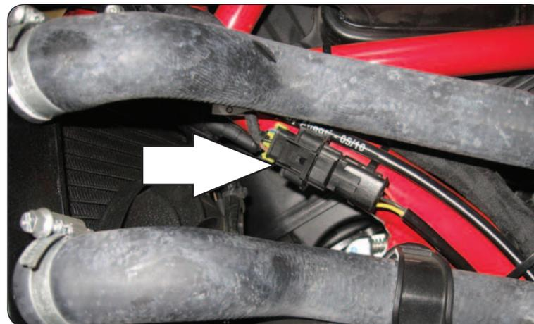
Figure B: Front coil connection
