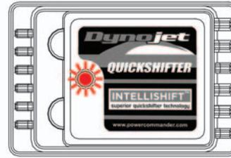
Move the gear lever to the trigger position 15 times, you'll see the status LED momentarily change to GREEN when the sensor is in the trigger position, then release the gear lever. Once you have moved the gear lever to the trigger point 15 times you'll now be able to count 5 RED status LED flashes. By doing this you'll have reduced the interrupt duration in RPM Band#1 by 10ms. (Remember, each RED status LED flash is worth 2ms)
