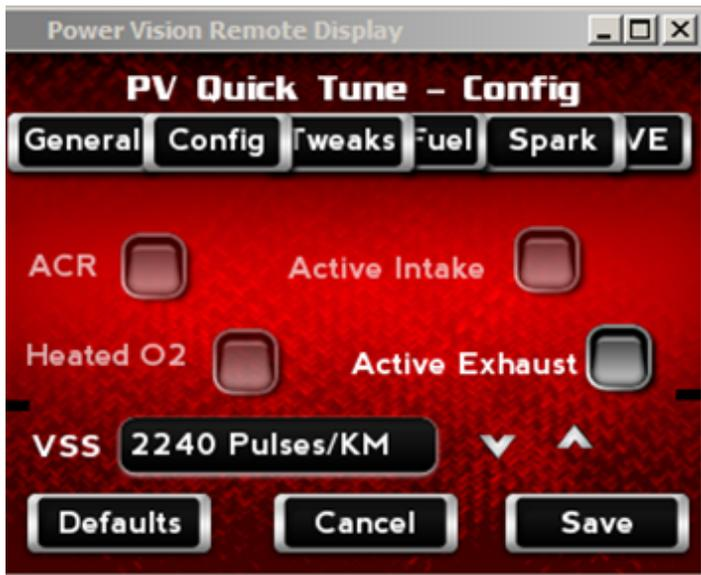
In Quick Tune (found under Program Vehicle), select the Config tab. See the VSS setting displaced here. This is the pulses per KM, or the rotations of the transmission output shaft in one kilometer. On the screen below the value is 2240. Your value will most likely be different.
