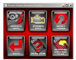
To start, with the Power Vision connected to the bike, select Vehicle Tools, **Restore Original Tune.**
