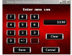
Next, flash any tune you want to use to the bike, and then go into **Quick Tune> Config Tab.** Change the VSS to match the value you noted earlier. You can use the up/down arrows to the right of the value, or press the value, clear, then enter the value needed. **Press Save, Save and go test.**
