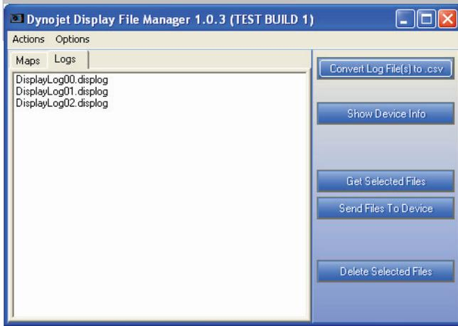
The Display File Manager software allows you to move log files between the Display and your computer. The main interface contains a set of tabs, Maps and Logs. These tabs display the files that exist on the memory card in the corresponding directory.
