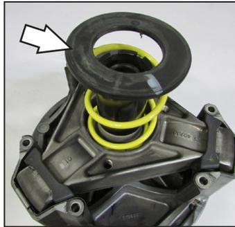
Remove the black plastic washer above the primary spring. **This spacer will not be reused.** Remove the clutch arms using 3/8" socket and 1/8" allen key. Install the Dynojet clutch arms with the proper amount of weight. Refer to chart on page 2. Install the Dynojet primary spring and reinstall the spring cover. Tighten the 6mm bolts evenly to 9 ft-lb (12 Nm).
