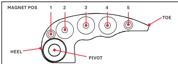
LOAD MAGNETS STARTING AT HEEL - POS #1
