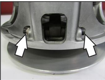
Remove the secondary clutch. Use a 15mm socket to remove the retaining bolt. Remove the snap ring and slide the secondary clutch off the input shaft. Before taking
